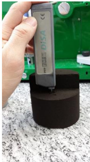
Figure 8: Digital durometer for mould strength measurement.
